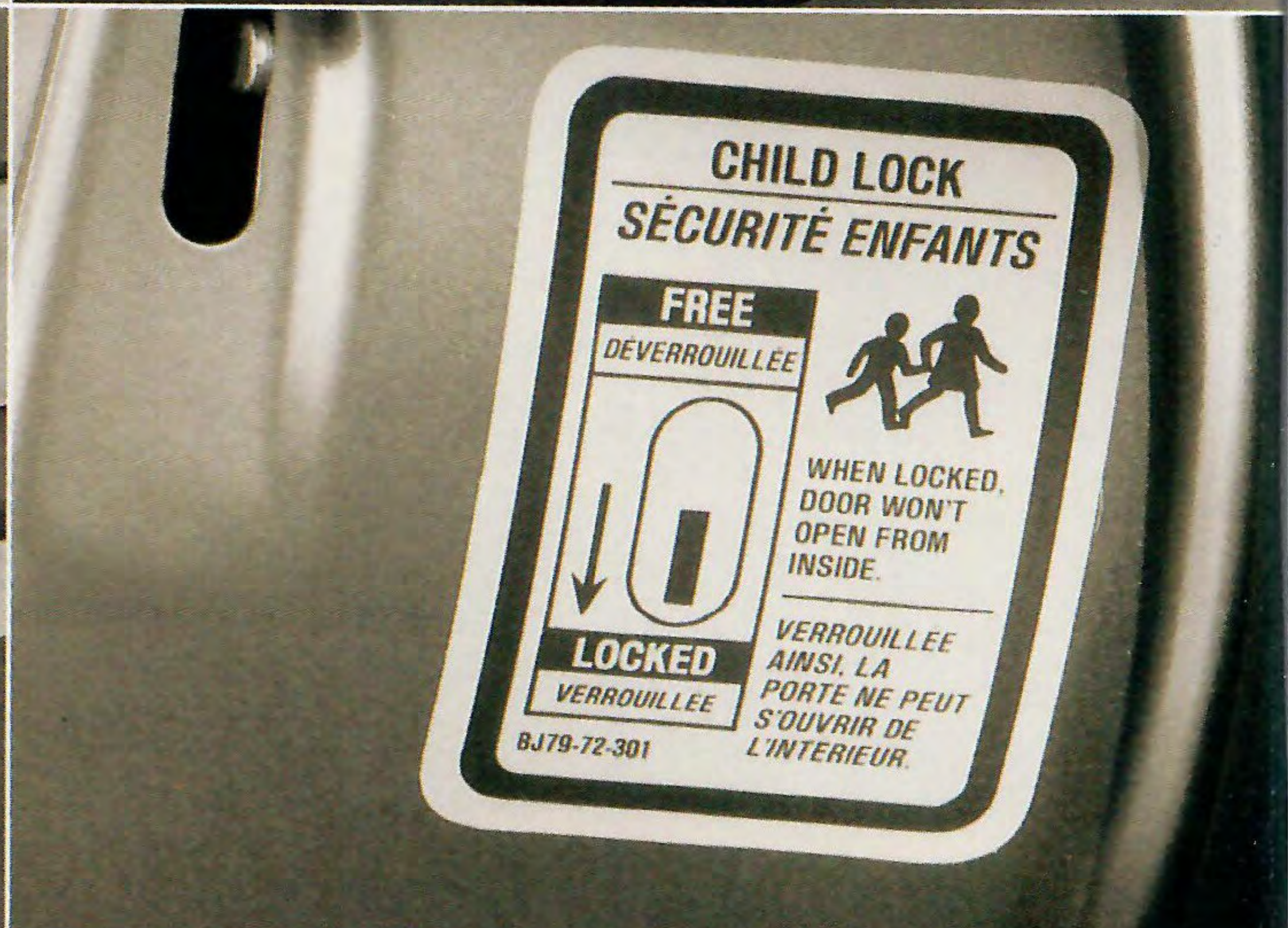
Child-proof door locks in the rear doors of all Mercury sedans as well as Villager keep children in back from accidentally opening the doors from inside the car, while allowing parents to still open doors from the outside.
